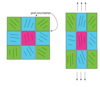
The strain is one crystal, shown in red, is also the strain in the whole polycrystal, as it is measured in the laboratory. We may now consider deformation in a one crystal as a unit problem for analyzing high temperature deformation in a polycrystal.
