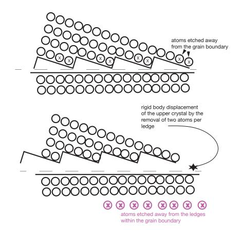
In this schematic, atoms marked by a cross are etched out of the grain boundary (and transported to the transverse boundary). This removal of these atoms is then accommodated by the two crystals moving closer to one another. The opposite would happen if atoms were to be inserted into the grain boundary - that would cause the crystal to move apart by rigid body motion.
