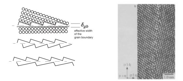
The structure of grain boundaries is illustrated by the schematic on the left and the high-resolution image obtained from transmission electron microscopy on the right. Note how the crystals extend into the grain boundary in the form of ledges. While these ledges can have different configurations, in all instances they provide sites where atoms can be added or removed.
